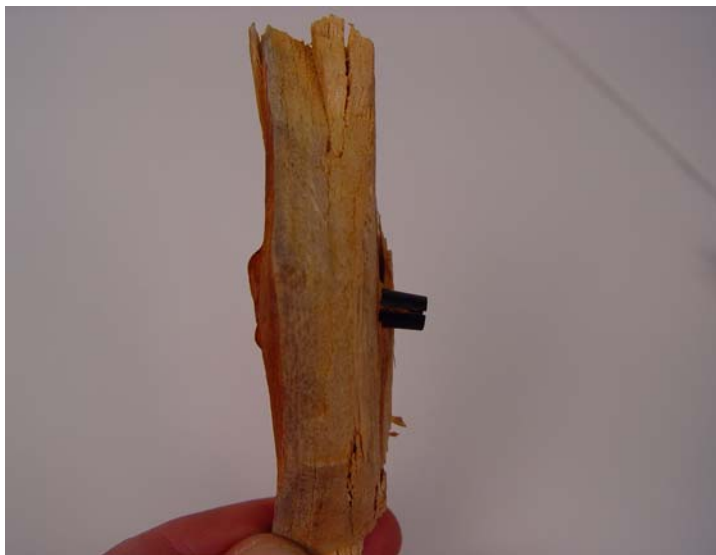
Figure 29. Excised Arborjet Injection Site two years following treatment, radial view. Note embedded Arborplug.
