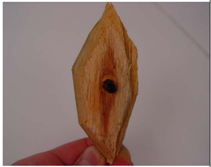
Figure 30. Tangential view of injection site showing limited reaction zones associated with buffered Phospho-jet solution.
