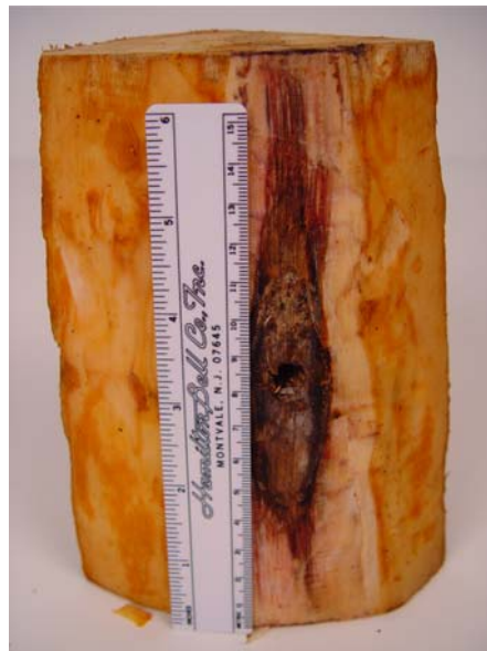
Figure 15 Same sample, as above with bark removed. Illustrates hypersensitivity in axial (wall 1) and in circumference (wall 2).
