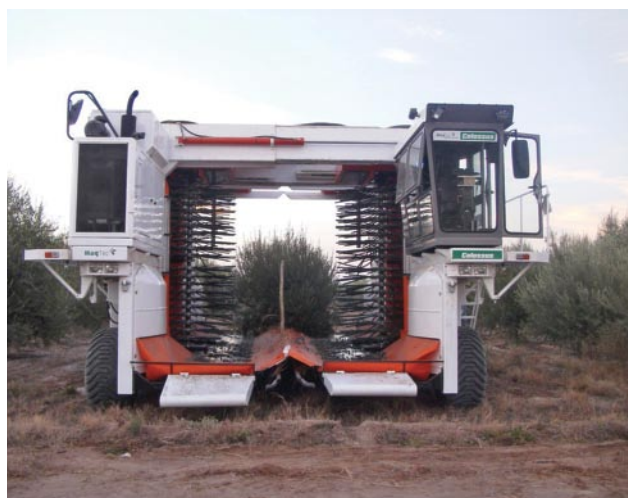
Mechanical straddle harvester for large scale harvesting of olives (Photo: Boundary Bend Estate)
