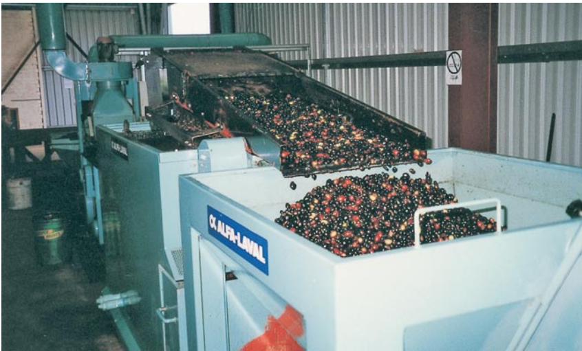
Washing fruit on a continuous process system
